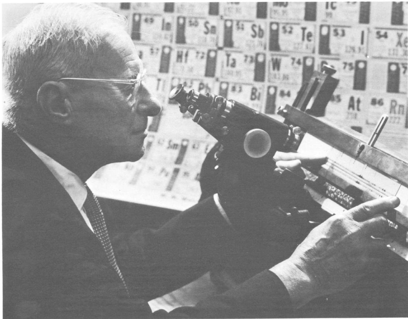
W. F. Meggers prepares to measure one of the spectrograms on which these tables of spectral-line intensities are based.
