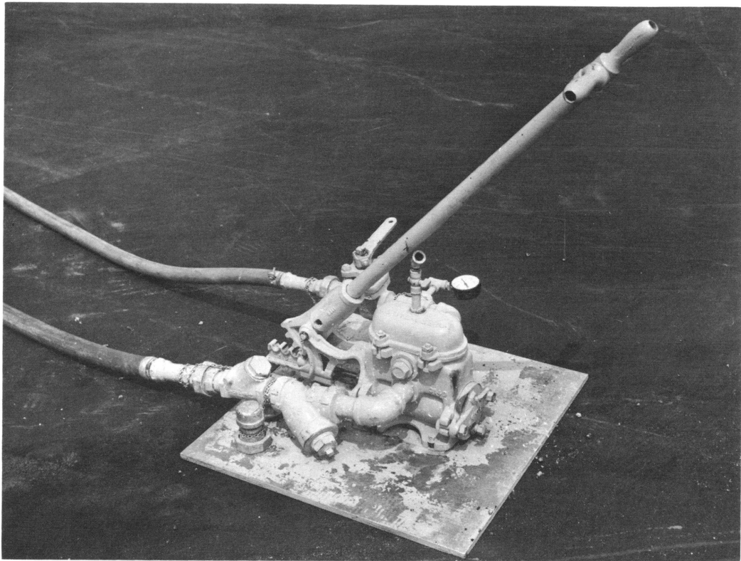
Fig. 2.8—Emergency hand pump.
