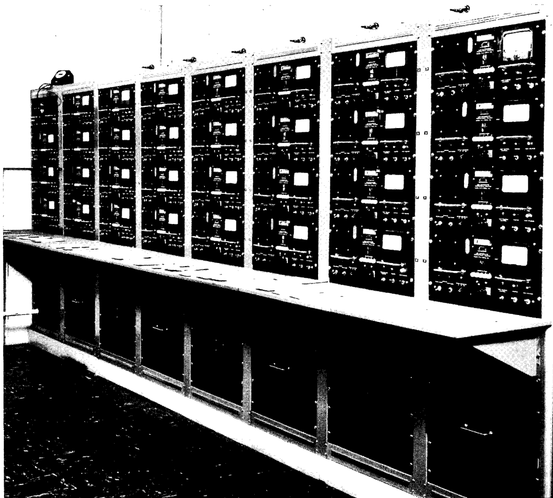
Figure 2. Urinalysis plate proportional counters.
