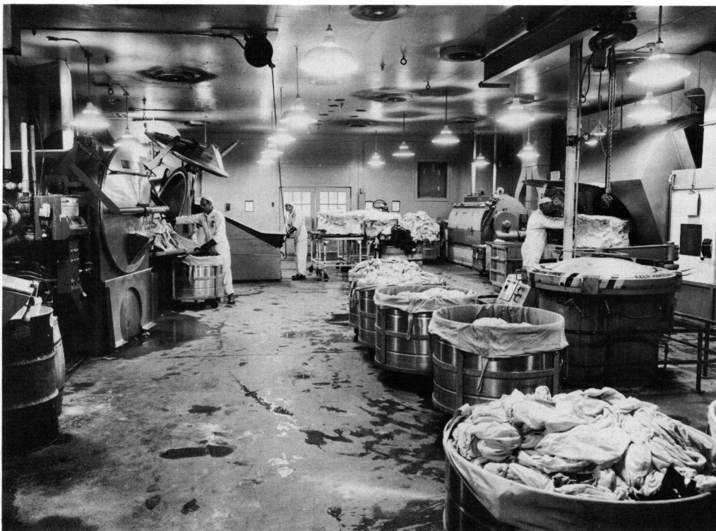
Figure 1. Wash room area with washer on the left, hydraxter in right foreground, and dryer in right background.
