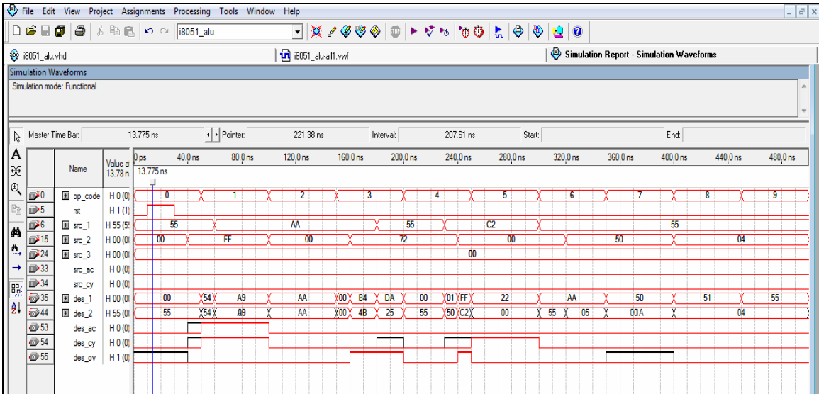
Figure 4.6-9: Comparison Report of Simulation of 8051 ALU Operation (Dalton Model with Verilog Model) for Op-Codes 0 to 9h
