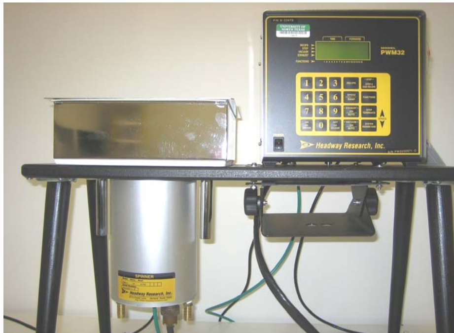
Figure 12: Spin coating set-up in laboratory.
