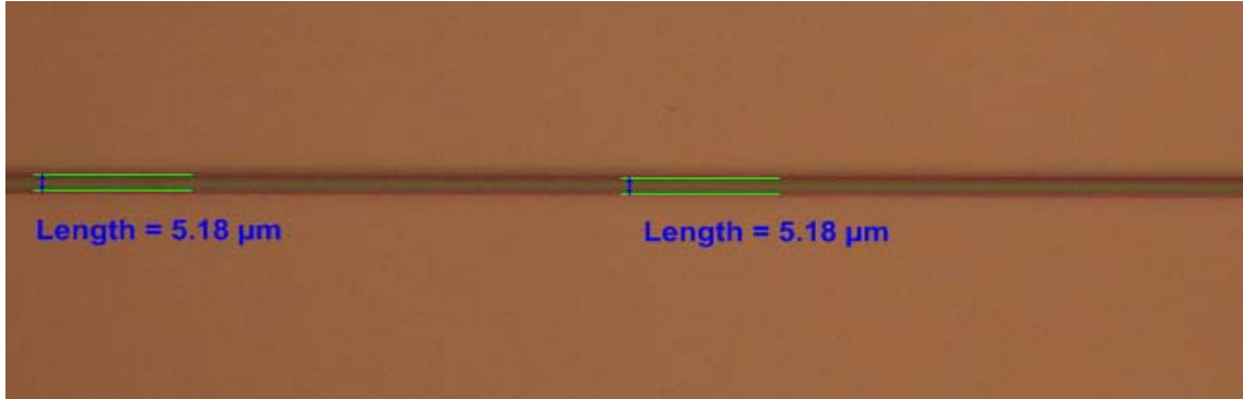
Figure 24: SU-8 waveguide with width of 5 microns.
