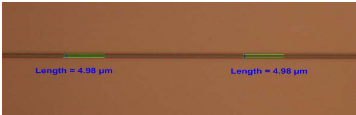
Figure 25: SU-8 waveguide 5 microns wide.
