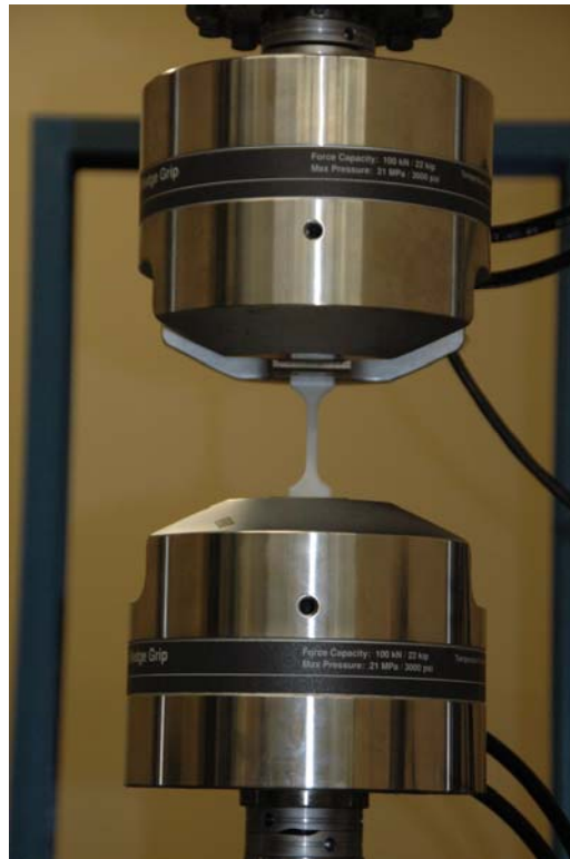
FIGURE 4.1. Dog-bone shaped specimen of UH mounted in the tensile testing Material Test System. The sample is shown at the start of the test before elongation.
