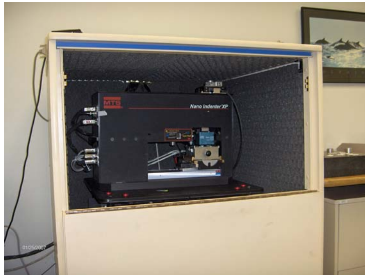
Figure 4a: Nano XP system (Nanoindenter™ manual, MTS Corporation [24]).
