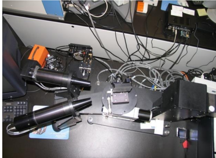
Figure 4.3 The commercially available ellipsometer used in measuring the refractive index of the hydrogel.
