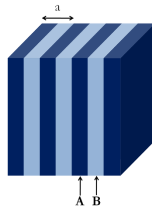
Figure 6.1 A one-dimensional photonic crystal comprised of the dielectric materials A and B, with a periodicity of a .
