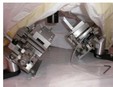
Figure 8.4 The 3-axis stages used for manipulating the photonic crystal and monomer.
