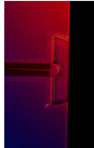
Figure 8.2 A close up of the lens structure used to focus the light onto the linear defect waveguide in the photonic crystal.
