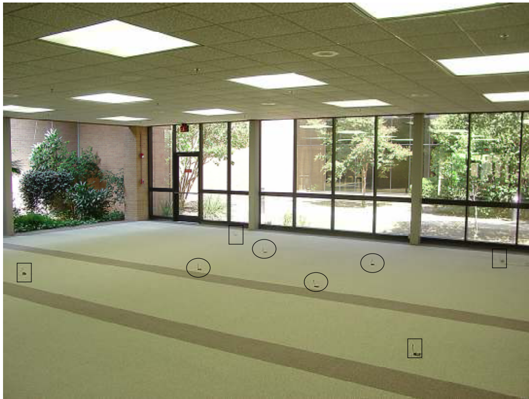
FIGURE 6.10. Experimental setup in the lobby near the south wing entrance of the College of Engineering at UNT. The circles in the indoor environment depict location-unaware sensor nodes and the boxes show the reference nodes deployed on the border.
