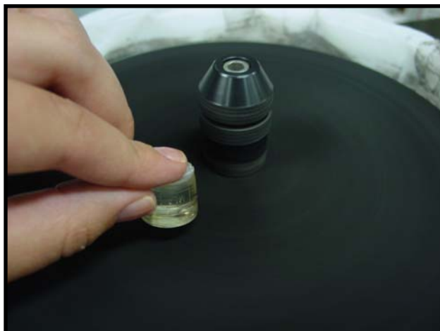
Figure 1-7 Fine grinding without the aid of lapping fixture.
