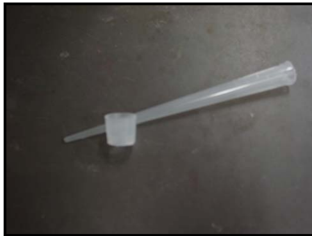
Figure 1-3 Non-tapered end of an MLA pipette as electrode mold.
