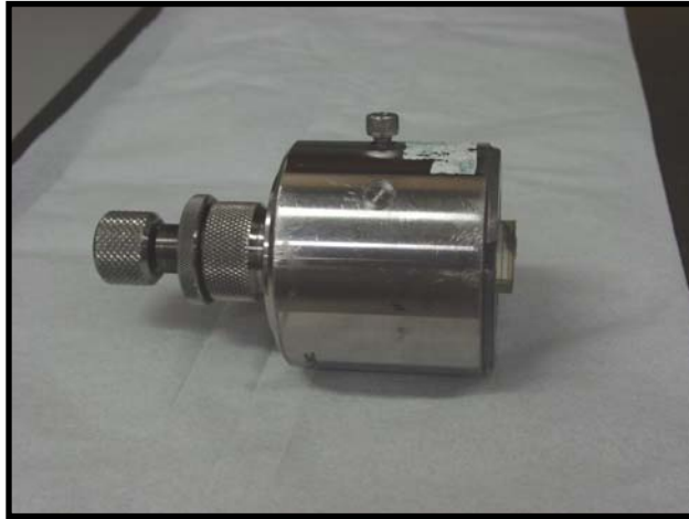
Figure 1-6 Electrode fixed in lapping fixture ready for coarse grinding.
