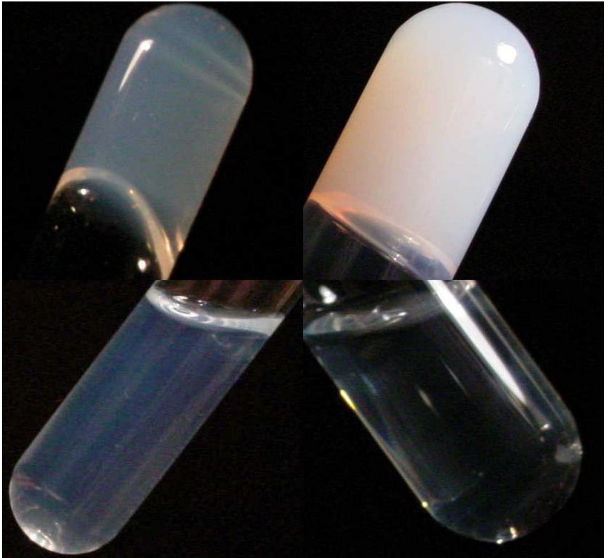
Figure 4.2: Images of IPN solution corresponding to phase diagram. From top left, clockwise, blue gelled, turbid gelled, clear flows, blue flows (~25°C for flowable images, ~37°C for gelled images).
