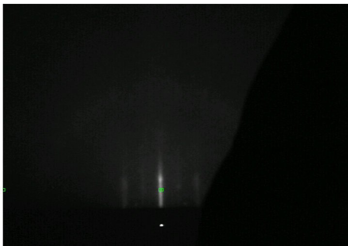
Figure 60. RHEED image after depositing Ge for 2 minutes.
