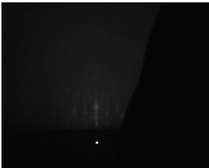
Figure 61. RHEED image at the end of depositing Ge.
