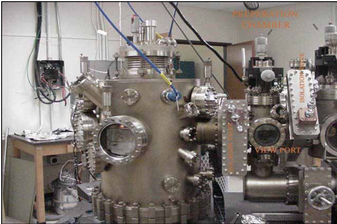
Figure 20. Preparation chamber of the III/V MBE system.
