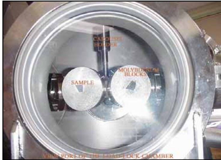
Figure 19. View port of the load-lock chamber showing the molybdenum blocks and samples.
