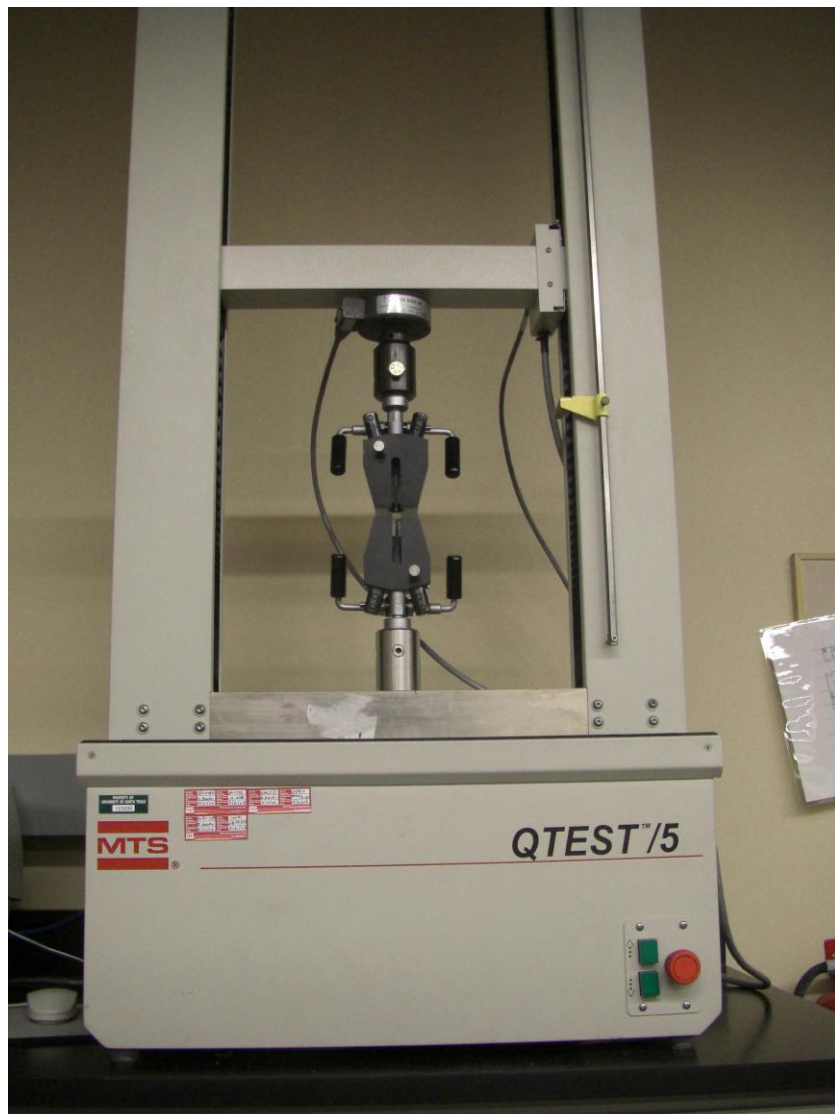
Figure 22. The QTEST/5 universal machine.
