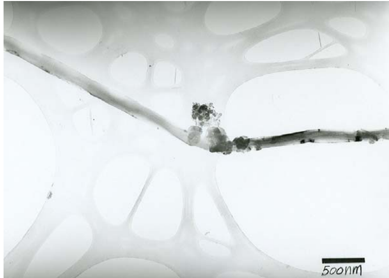
Fig. 2.3 A TEM micrograph of a MWCNT at a low magnification
