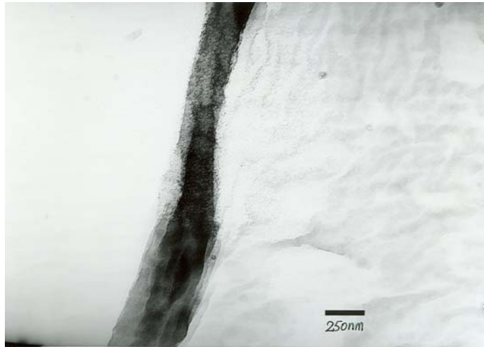
Fig. 2.1 A TEM micrograph of SWCNTs at a low magnification.
