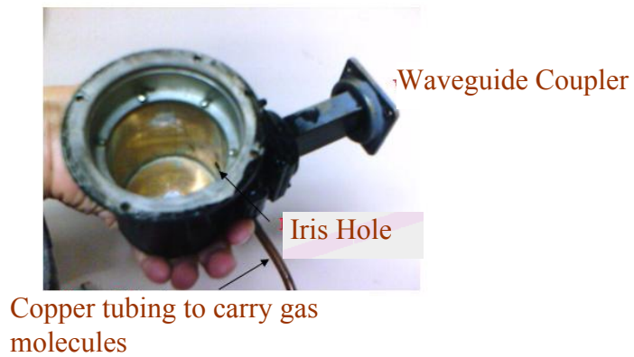
FIG. 17. An interior view of the bottom half of the cavity.
