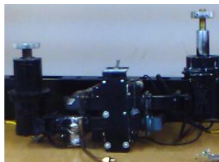
FIG.14a (left) and FIG.14b (right). Ring gauge and coupled resonant cavities.
