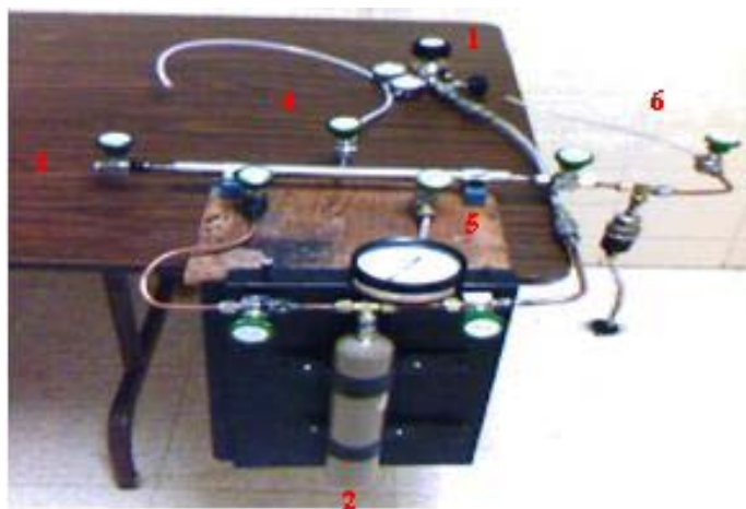
FIG. 13. Customized manifold assembly to regulate the flow of gas from high to low pressure.
