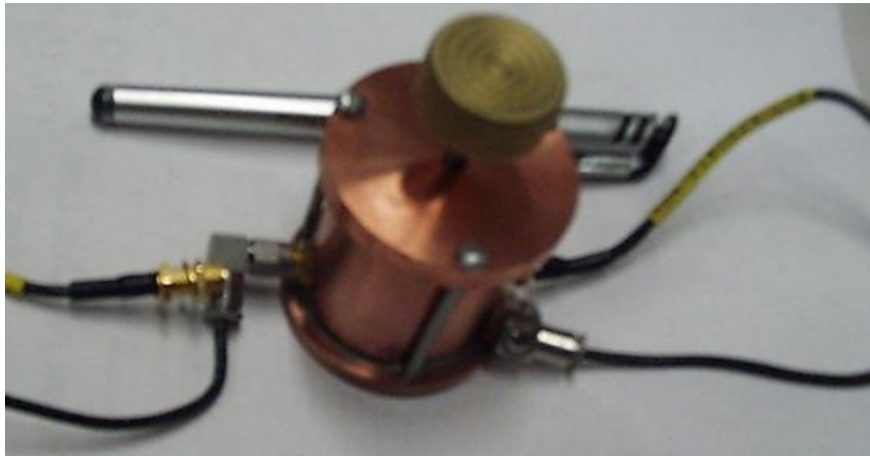
FIG. 52. A sample miniaturized resonant cavity to selectively detect toxins.
