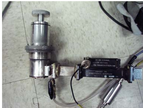
FIG. 16. Shown on the side wall of the waveguide is the feed in line on the opposite wall (not visible) and an output to measure the reflection profile of the signal.
