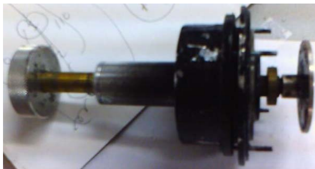
FIG. 19. A tuning rod for tuning the resonant cavity to a selective mode
