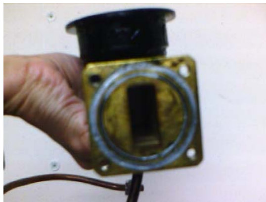
FIG. 18. Coupling of the waveguide to the sidewall of the resonant cavity along its long dimensions parallel to the axis of the cavity.
