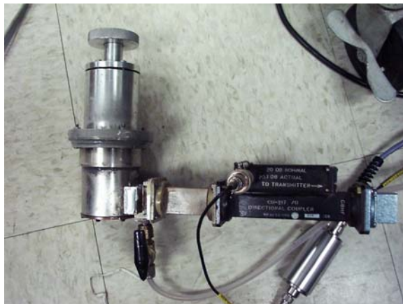
FIG. 2. A picture of the typical resonant cavity with the gas connector cables and the waveguide coupling through the iris hole.
