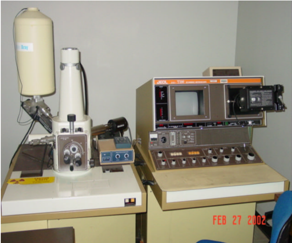
Figure 3.3 JEOL model JMS-T300 Scanning Electron Microscope. The microscope was used to inspect the quality of tip etching.
