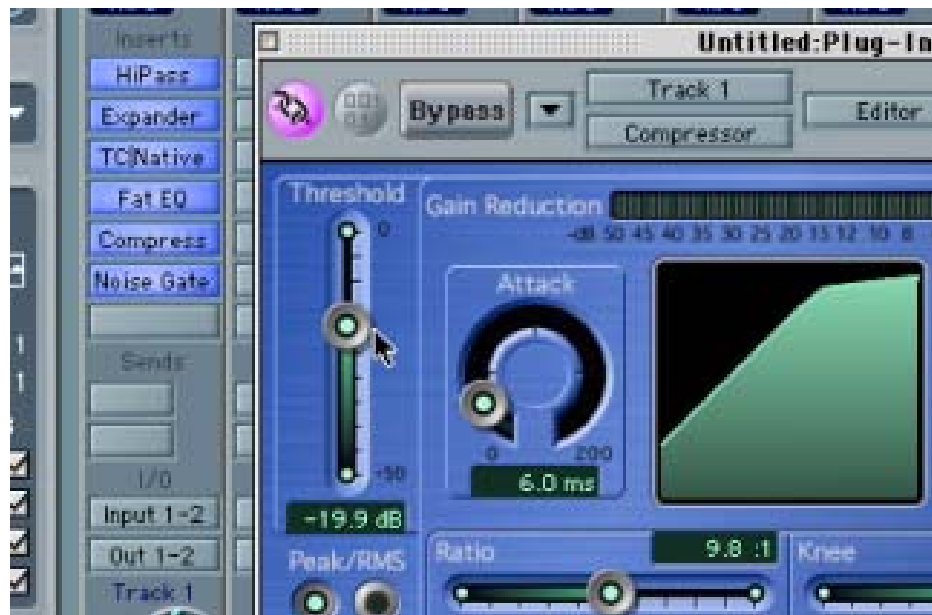
Fig. 6. Combination of compressor, expander, and equalizers plug-ins used for noise reduction.
