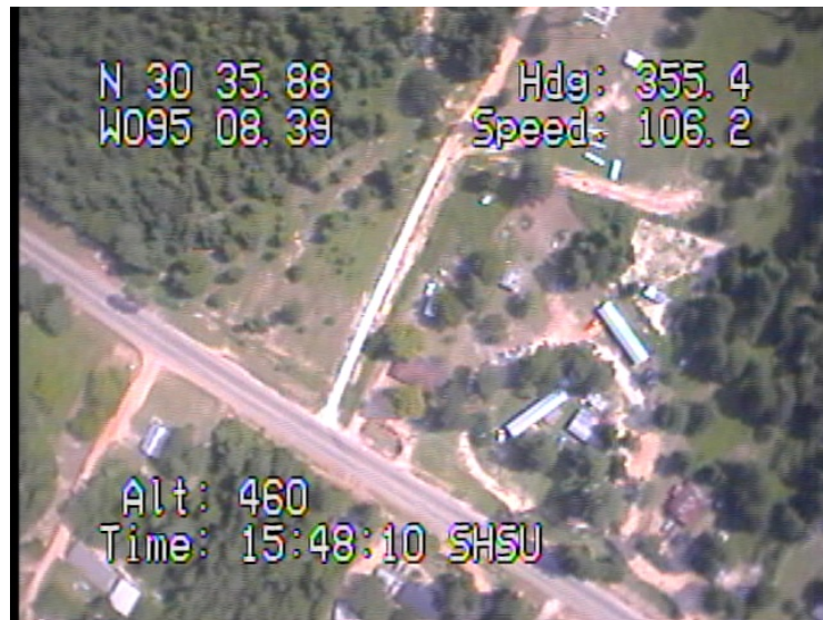
Figure18. The aerial video frame with serial data overlay.
