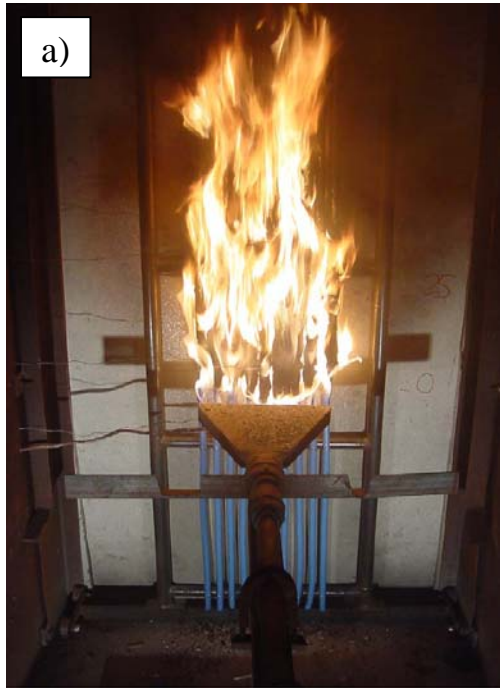
Figure 3 a) The fire model in action, and b) a cable ladder after burning
