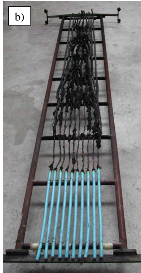
Figure 3 a) The fire model in action, and b) a cable ladder after burning
