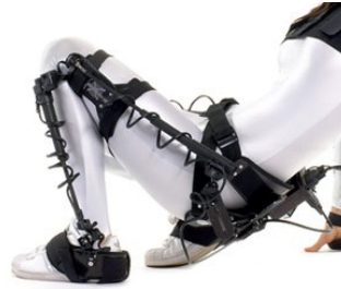
Fig. 19 – Motion capture exoskeleton
