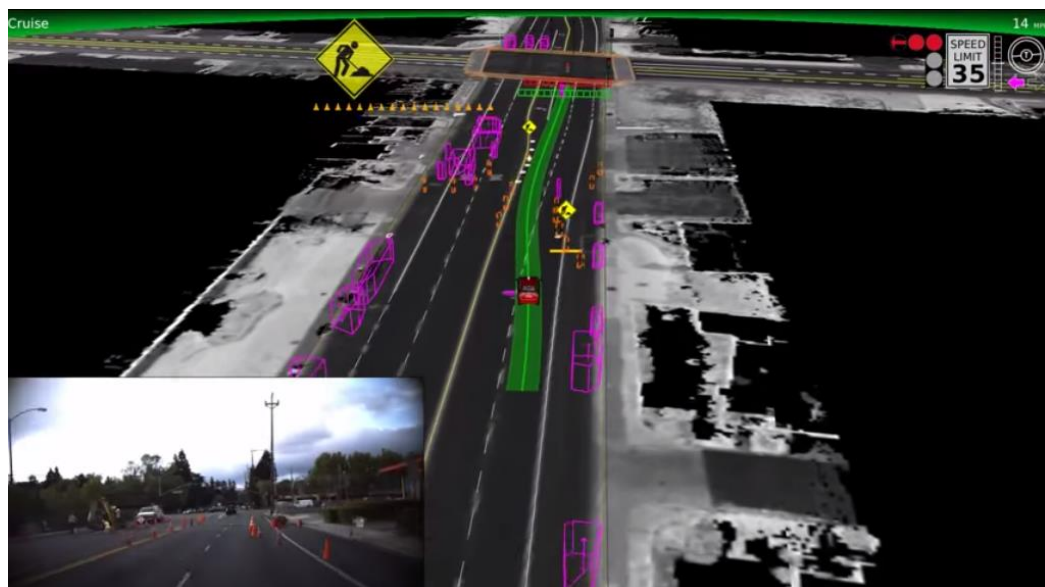
Figure 2-2: The sensors and camera recognize objects on the streets such as road signs, other vehicles, pedestrians and cyclists. Source: Urmson (2014)
