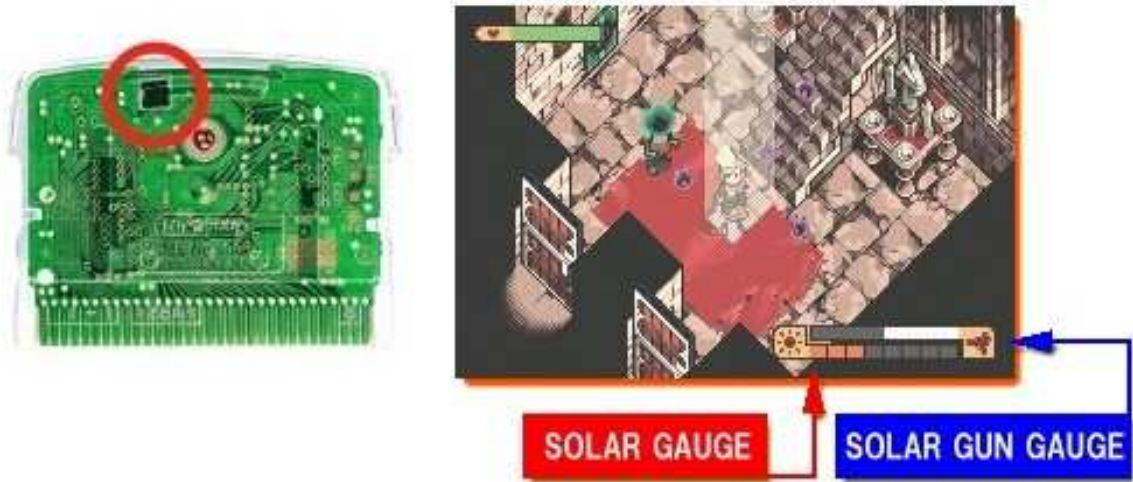
Figure 15 – Left: Boktai: The Sun is in Your Hand 's cartridge. The circle points out the solar sensor. Right: Screenshot from the game.
