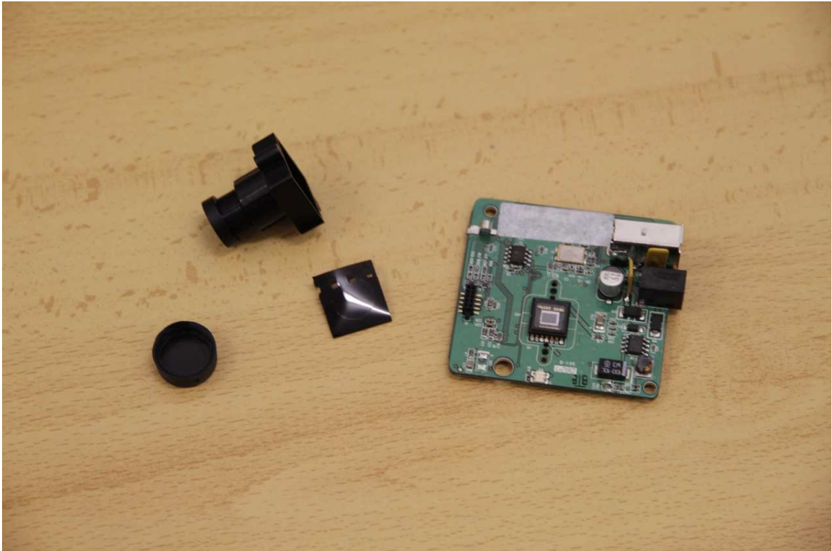
Figure 28 – Our Unibrain Fire-I without the lens support and the film square we used as an IR filter. (Photograph by the author)
