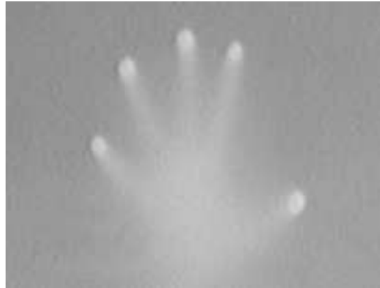
Figure 27 – An example an image produced by a rear DI multi-touch table. (Retrieved from http://wiki.nuigroup.com/Diffused_Illumination on 20/04/2012)
