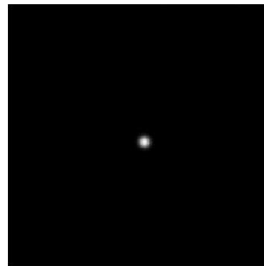
Figure 4.29. Binary image obtained from the Matlab code by using the processed list mode data. The cylindrical source was placed in the centre of the patient table
