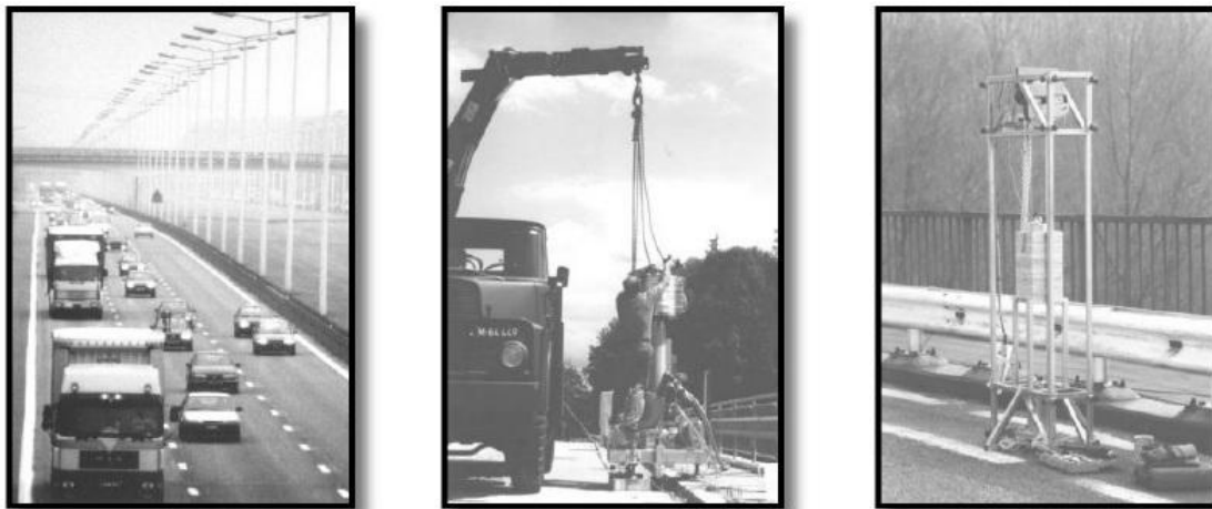
Figure 5-2: Excitation Sources of the Z24 Bridge: on the left the highway traffic, in the middle the installation of a mass shaker and on the right the drop weight system.
