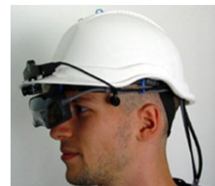
Figure 2 - HMD (source: Carmigniani et al (2011). Augmented reality technologies, systems and applications)
