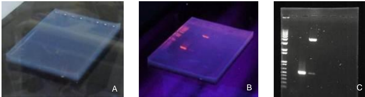
Figure 1.6: Representation of an agarose gel observed at naked eye (1.6 A), a digital image of the same gel (1.6 B) and the gel transilluminated with UV radiation (1.6 C) (In: Henriques, 2011).
