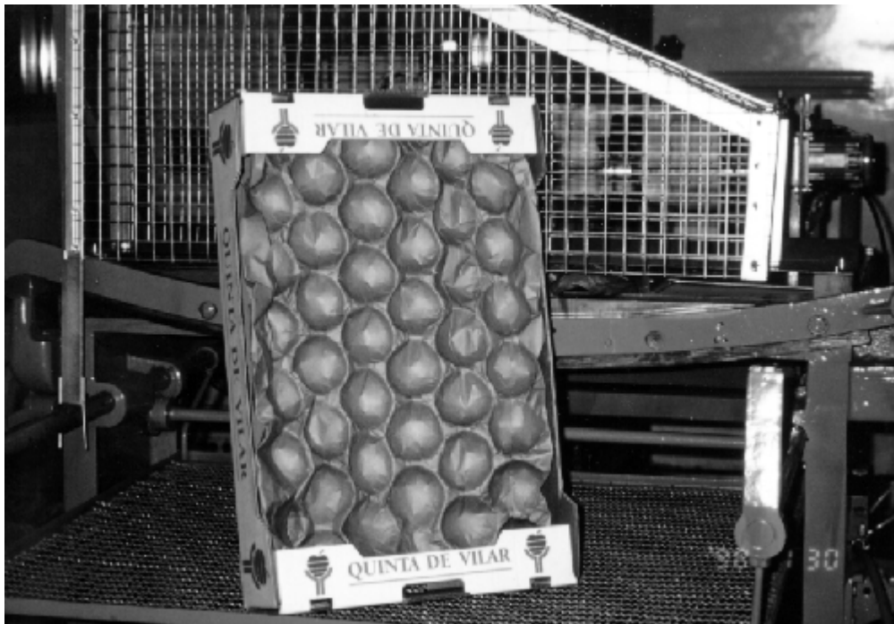
Figure 3a. Moulded paper tray inserted in corrugated transportation tray.
