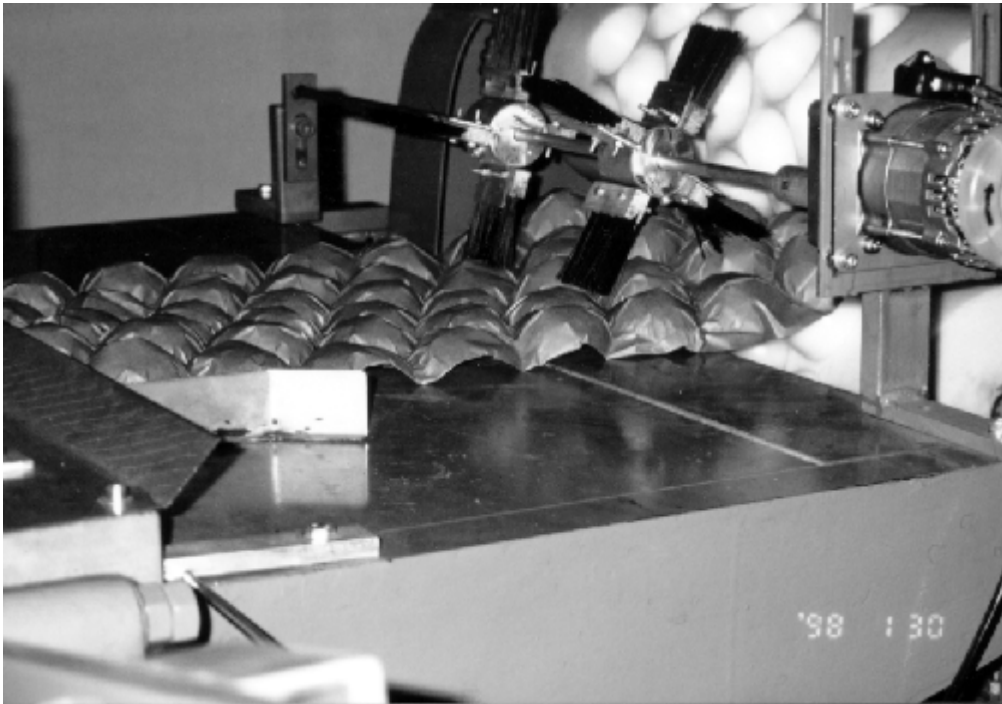
Figure 6. Paper web extraction after moulding.
