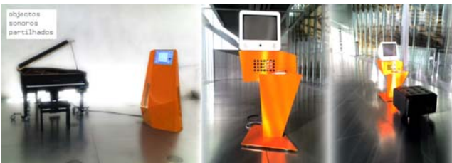
Fig. 2 The PSOs Server connected to the Disklavier Piano and two of the clients which remotely control the same Piano
