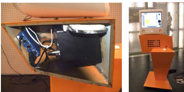
Fig. 3 A PSOs Client with the ETHERSOUND Hub, Speakers and Keyboard concealed on the structure.
