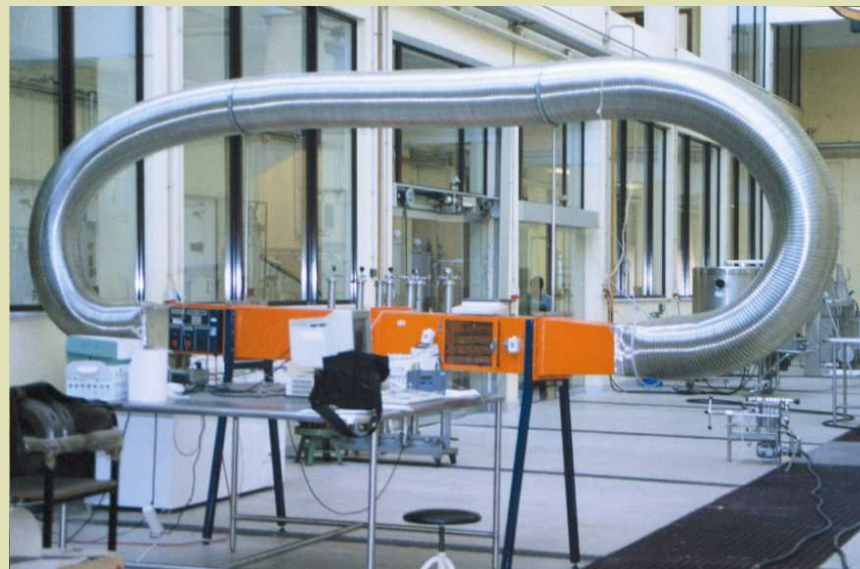
Pilot plant convective tray drier (Armfield UOP8).
