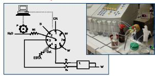
P – peristaltic pump; SV – selection valve;  $\lambda$  – spectrophotometer at 543 nm; HC – holding coil (30 cm); Col. – cadmium column;  $R_{\rm l}$  – reactors; CR – colour reagent (sulphanilamide 20 g/L, N1NED 2 g/L in  $H_3PO_4$  1.5 M ); S – sample or standard; EDTA – conditioner (EDTA 0.55 g/L with NH $_4$ Cl 21 g/L); W – waste.
