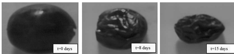
Fig. 1. Macroscopic shrinkage of grapes during drying (Ramos, 2003).
