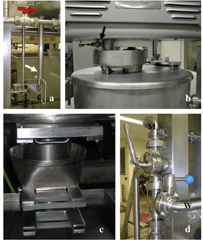
Fig. 2. Building details of the novel cheesemaking apparatus: (a) periscope for drainage (white arrow); (b) upper end of cheese vat, showing the lid with opening used to add the (plant) rennet, and the detector that determines the position at which the stirring/cutting frame is to rest when the motion is stopped (black arrow); (c) perforated cylinder, inside which pre-moulding of cheese takes place; and (d) inlet tubes, through which milk (M) and water for cleaning (W) are admitted into/out of the cheese vat.
