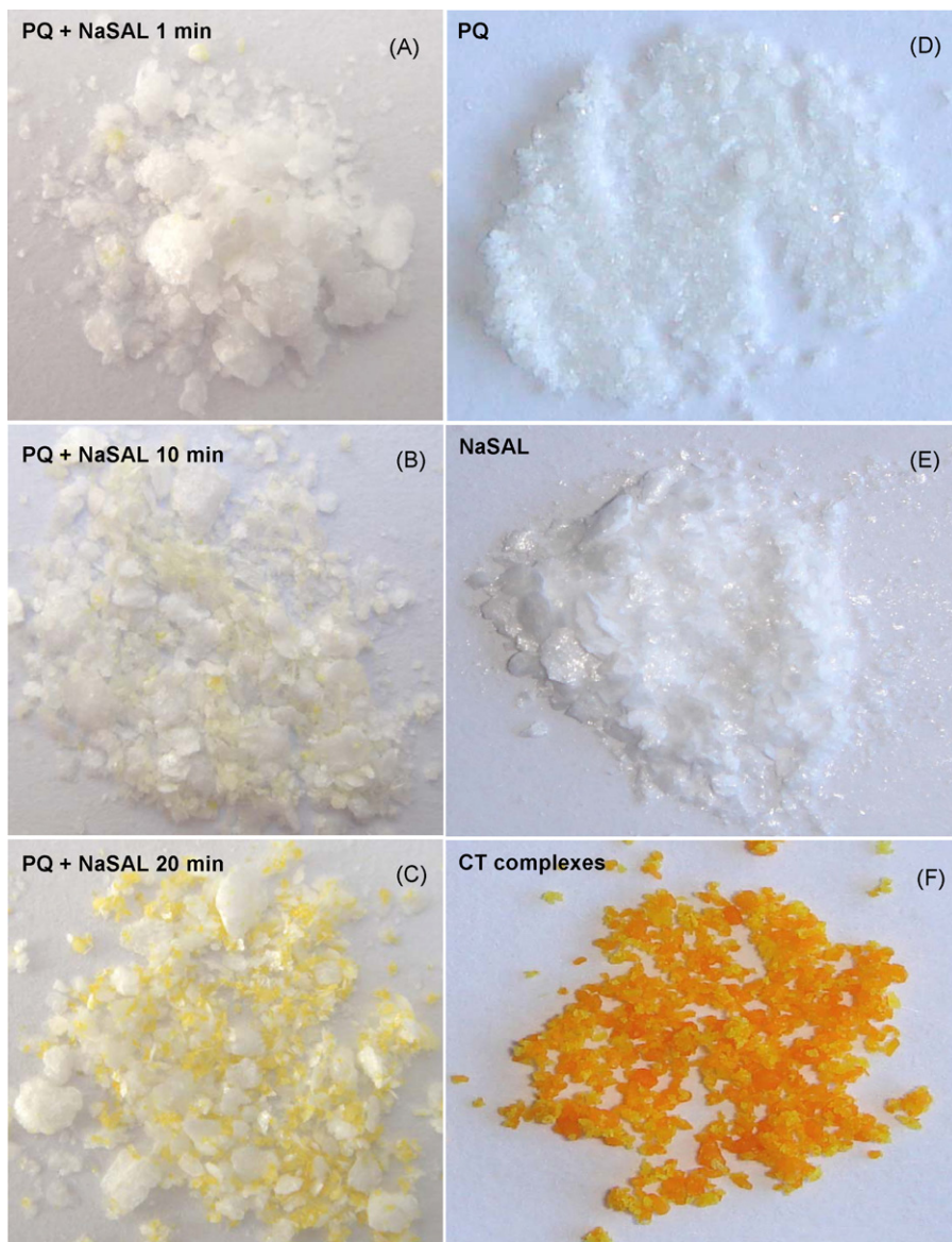
Fig. 2. Photographs of the time-course reactivity of paraquat (PQ) and sodium salicylate (NaSAL), 1 min (A), 10 min (B) and 20 min (C) after mixing both powders. Photographs of PQ (D), NaSAL (E) and of the charge-transfer (CT) complexes (F) recovered as solids according to the method described by Ledwith and Woods (1970).
