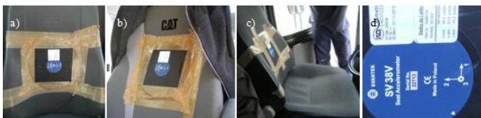
Figure 2. Placement of the whole-body accelerometer in the seat backrest of the a) rock drill, b) shovel and c) dumper.
