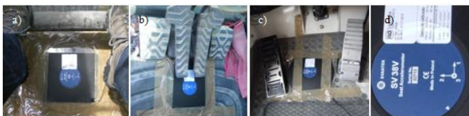
Figure 3. Placement of the whole-body accelerometer in the cabin floor of the a) rock drill, b) shovel and c) dumper,
