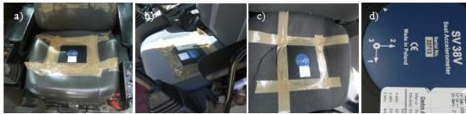
Figure 1. Placement of the whole-body accelerometer in the supporting seat surface a) rock drill, b) shovel and c) dumper.
