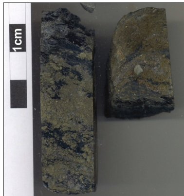
Figure 1. Hand specimen sample of gold-rich banded black shales with pyrite. Massive pyrite dominates the mineralogy at the hand specimen scale. (Borehole sample LOU08/01-7).
