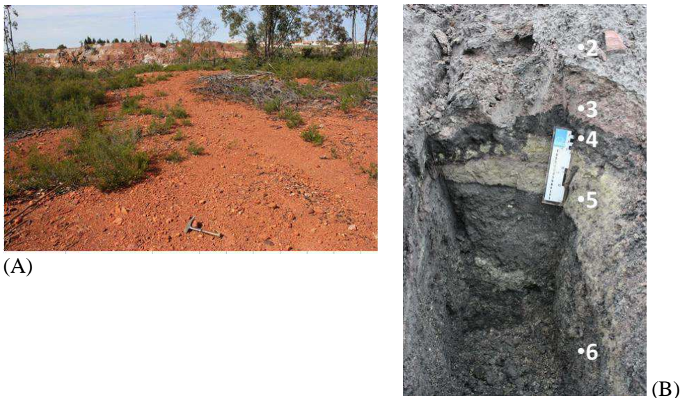
Figure 1 (A) Milled gossan dump located in the southern part of the São Domingos open pit; (B) Profile in the waste pyrite ore ash pile at Achada do Gamo sulfur production area.
