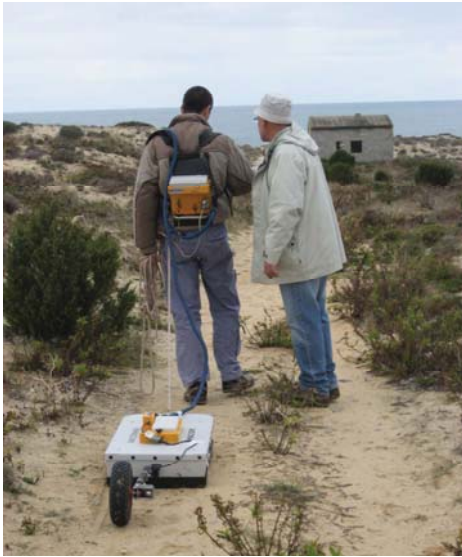
Figure 3 - Equipment used in the acquisition of the GPR profile.
