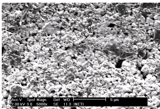
Fig. 3. SEM micrograph of the fresh cathode sample (in charged condition).
