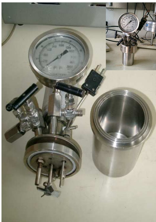
Fig.1 Stainless steel (type 316) reactor used for the study of sodium borohydride catalysed hydrolysis, under pressure up to 70 bar.
