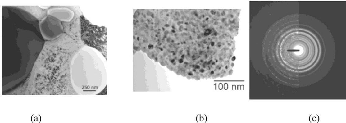
Figure 2. TEM investigation showing the nanocrystalline structure: (a) bright field image of the solution treated material; (b) bright field image and (c) SAED pattern of the NiTi matrix of the aged material.
