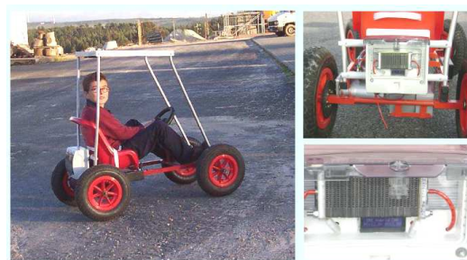
Figure 8 Kid Kart and implemented hybrid fuel cell system.
