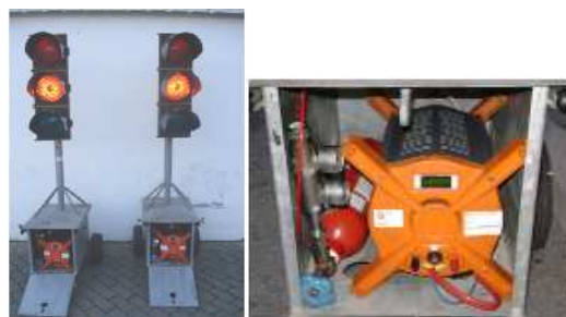
Fig.2 Traffic Lights Demonstration Project showing fuel cell and hydrogen storage.
