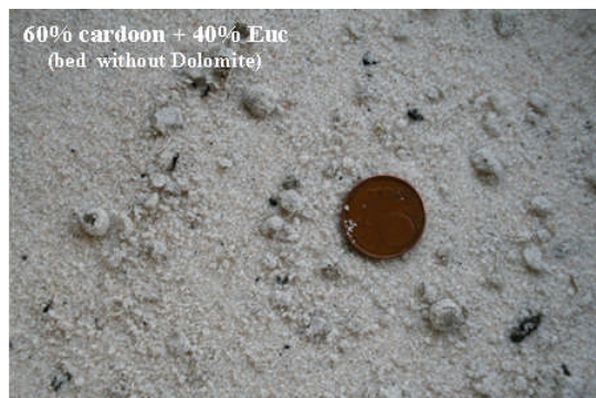
Fig. 5 Small agglomerates formed during combustion of 60%Cardoon+40% Eucalyptus; Tbed=730°C
