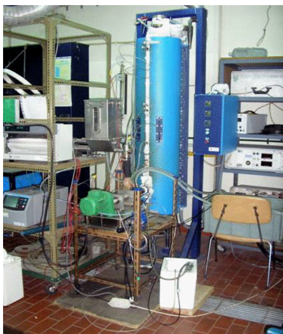
Fig. 1 Bench-scale combustion installation
