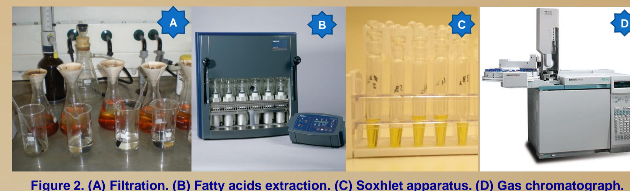
Figure 2. (A) Filtration. (B) Fatty acids extraction. (C) Soxhlet apparatus. (D) Gas chromatograph.
