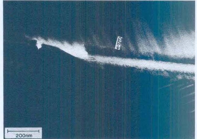
FIG. 10. Sample sintered at 970 °C in 0.5% CO 2 + 99.5% O 2 . TEM micrograph for the grain boundary, as marked by G.B., which is wet by a layer of BaCuO 2 second phase.
