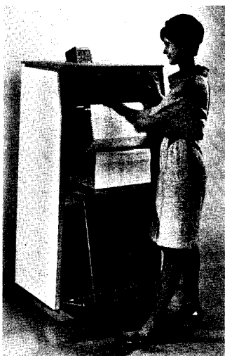
Fig. 2. Recordak Rotoline Microfilmer. Unburst paper output is recorded on film.
