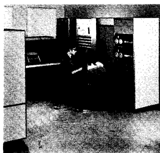
Fig. 4. Information on a Microfilm Frame is Scanned and Converted to Digital Form by a Unit Such as the Information International PFR-3.
