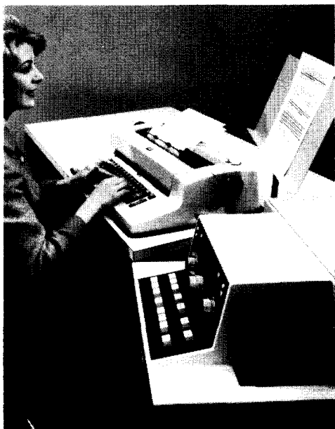
Figure 1. A Typist at the Keyboard of the IBM Magnetic Tape "Selectric" Typewriter (MT/ST).
