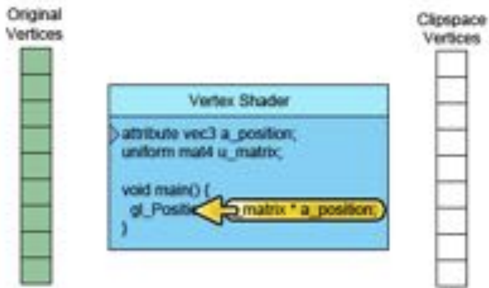
Figure 2-6: WebGL vertex shader that shows 9 vertices being processed
