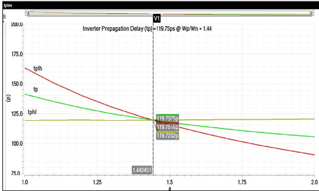
Figure 4.8: Propagation delay waveform of the designed inverter.
