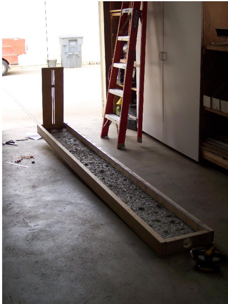
Figure 1. Dry ravel flume used in experiments.
