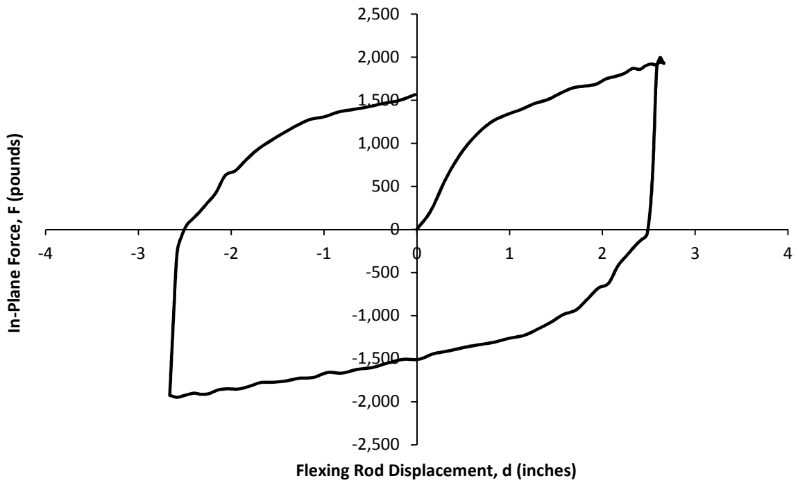
Figure 65. Force developed in the exterior flexing rod versus the exterior link displacement.
