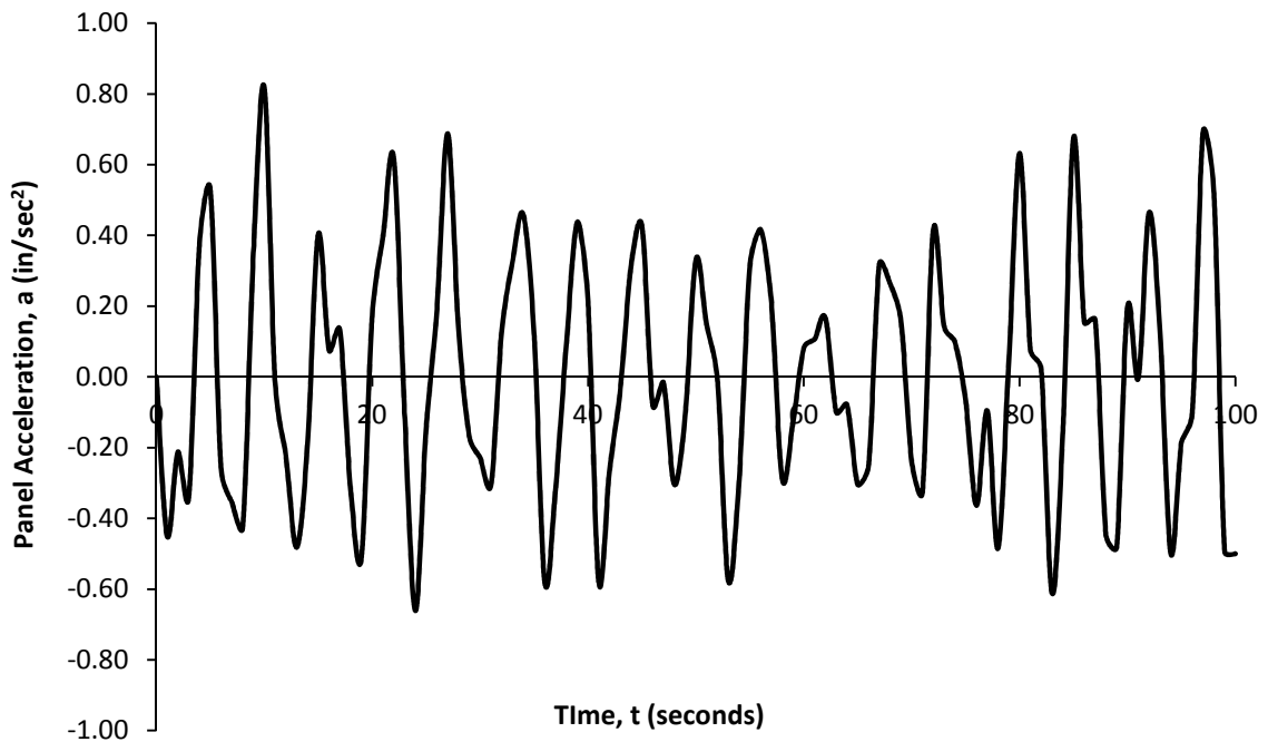
Figure 45. Precast concrete panel acceleration in the X direction versus time.
